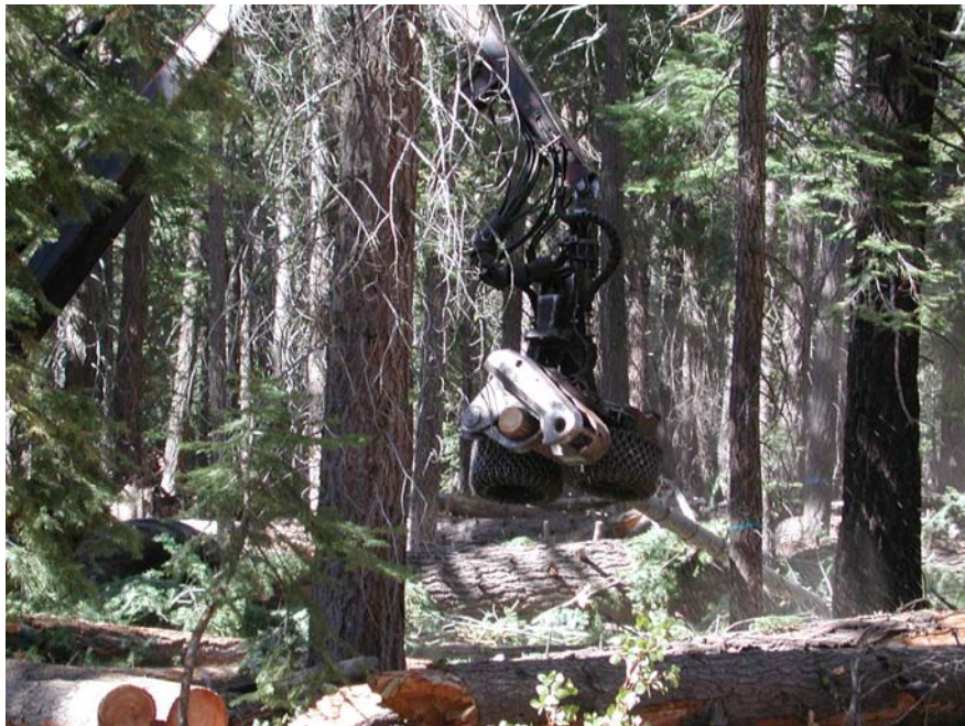
“Cut to length” operation for fuel reduction
