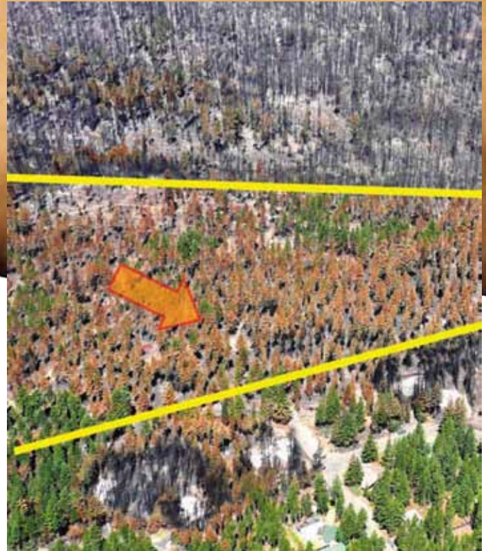
Element of a Fire Adapted Community: A high-intensity wildfire was burning through tree crowns (black area in the upper half of photograph) during the Lake Tahoe Basin's Angora Fire. The orange arrow shows the direction the fire was burning. When it reached a fuelbreak where the trees had been thinned, the fire changed from a crown fire to a lower-intensity surface fire (area of brown trees) that reduced the threat to nearby homes. Community fuelbreaks are often a key element of becoming a Fire Adapted Community. Photograph from "An Assessment of Fuel Treatment Effects on Fire Behavior, Suppression Effectiveness, and Structure Ignition on the Angora Fire," R5-TP-025, USDA Forest Service.
